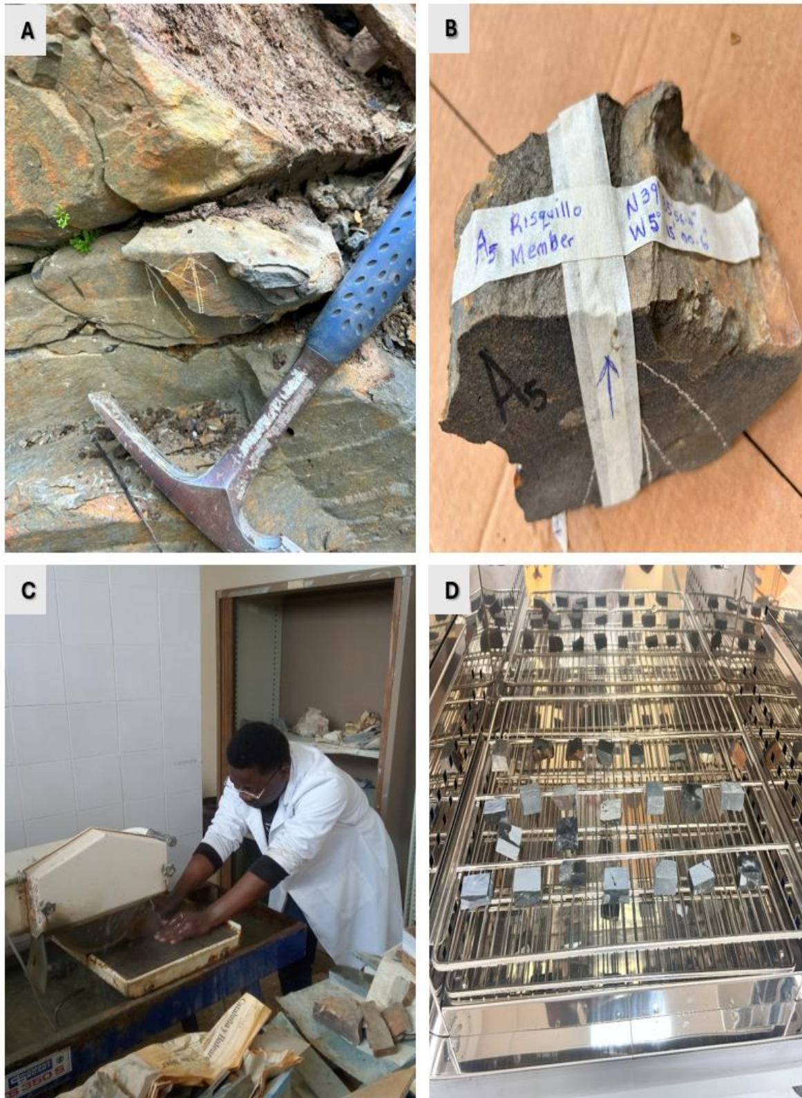
Figure 3. A and B, sample collection and marking for stratigraphic orientation. (C) Sample cutting process, and (D) Samples were placed in an oven for several hours to make sure there was no moisture left
